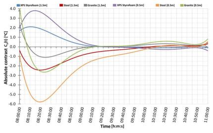
Fig. 5. Differences absolute contrast at two different levels of heating the surface (temperatures provided in the legend)
