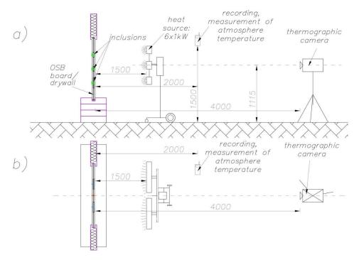
Fig. 2. Plan of test station applied in active thermography in the reflective mode
